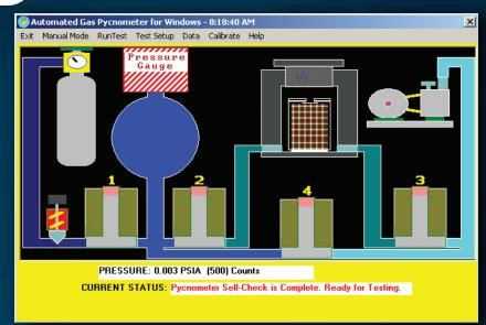
pycnometer measures the true volume and density of solid powders such as calcinated petroleum coke.
